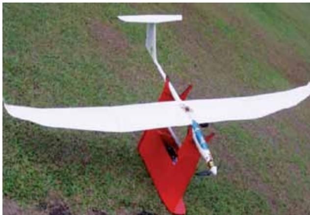
*Fig. 3: CropCam Unmanned Aerial Vehicle (UAV)*
