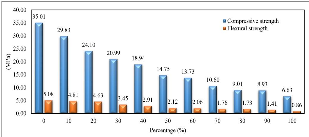
Figure 7. Variation of Modified-CKD for 7 days curing
