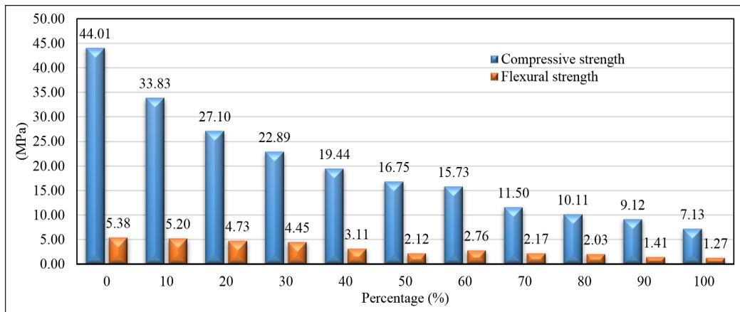
Figure 8. Variation of modified-CKD for 14 days curing
