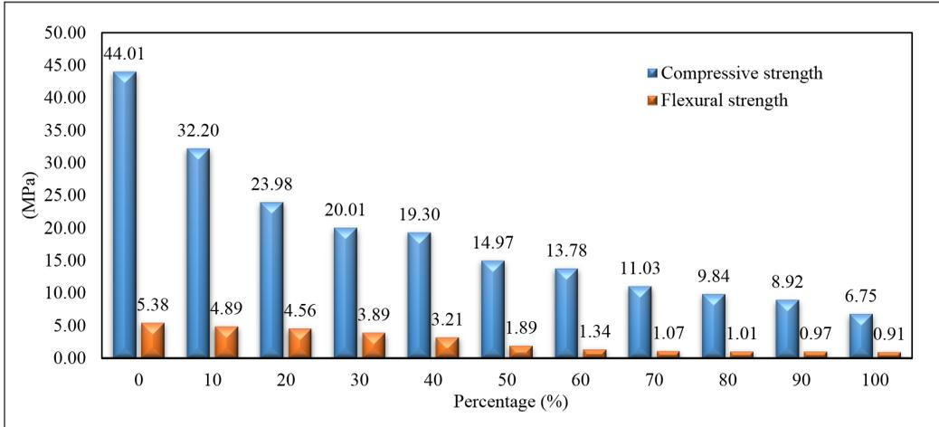
Figure 5. Variation of normal-CKD for 14 days curing
