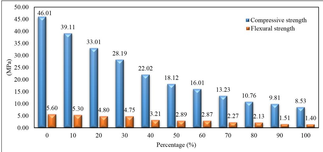
Figure 9. Variation of modified-CKD for 28 days curing
