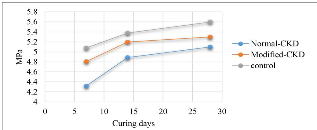
Figure 11. Flexural strength trends for 10% addition
