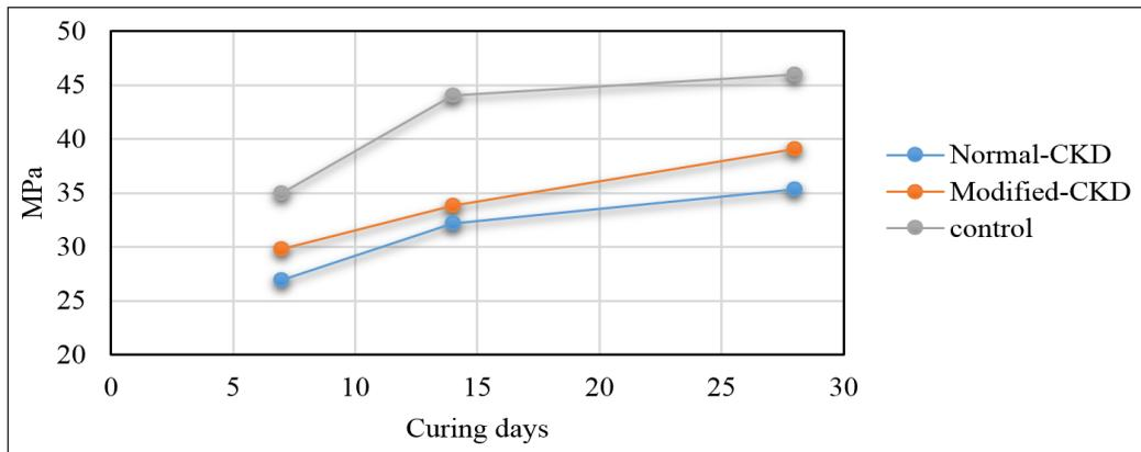
Figure 10. Compressive strength trends for 10% addition
