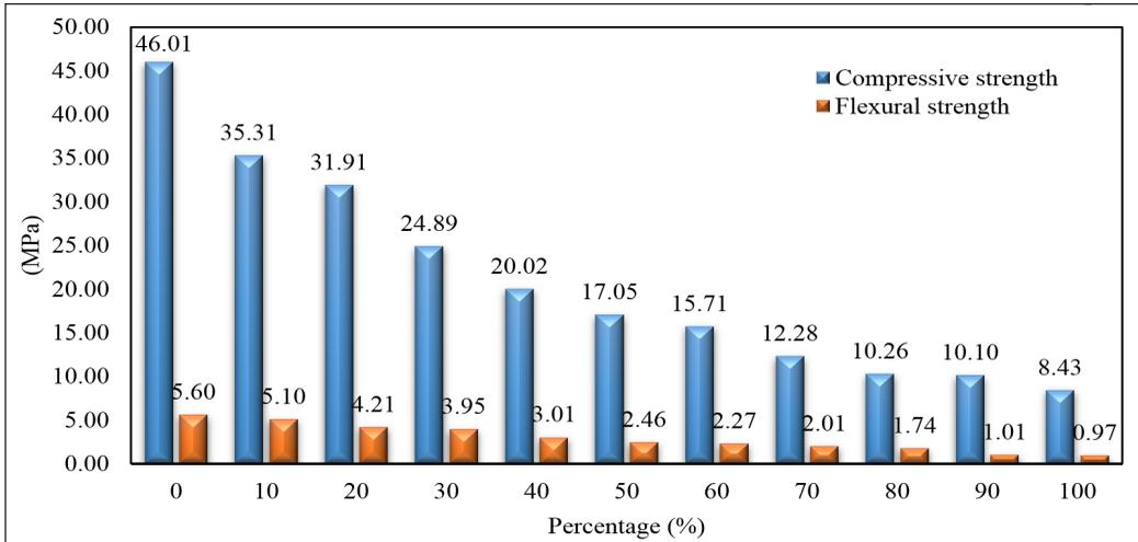
Figure 6. Variation of normal-CKD for 28 days curing
