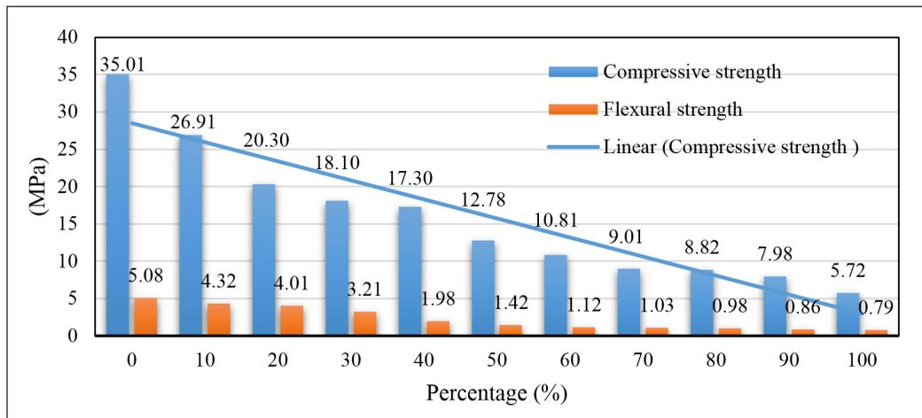
Figure 4. Variation of normal-CKD for 7 days curing
