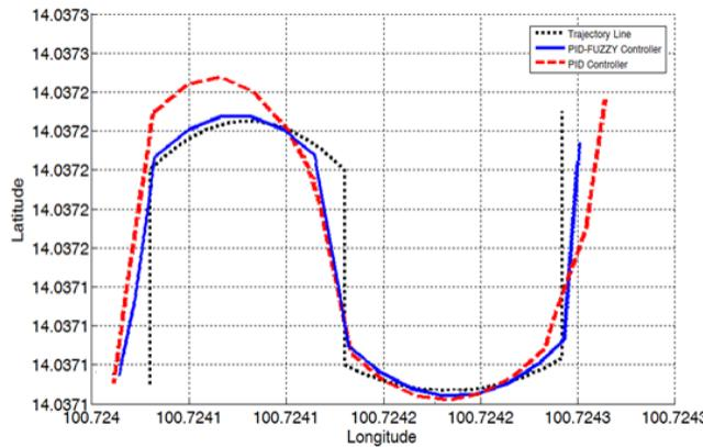
Figure 16. Experimental results of the N-shaped trajectory tracking control of the tractor
