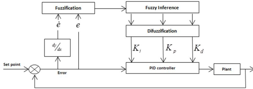
Figure 2. Self-tuning fuzzy PID controller
