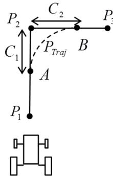
Figure 9. A curved line constructed from two straight lines
