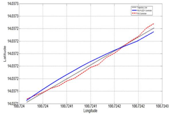
Figure 12. Experimental results of straight line trajectory tracking Control
