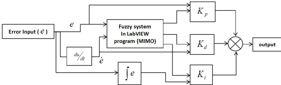
Figure 10. Block diagram of self-tuning fuzzy PID controller.
