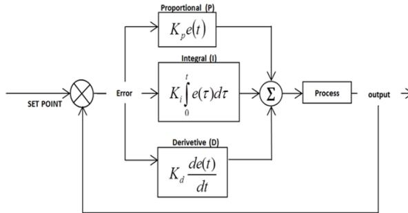
Figure 1. Block diagram of the PID controller
