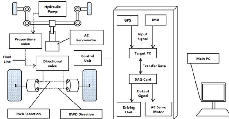
Figure 5. Working Diagram of Autonomous tractor
