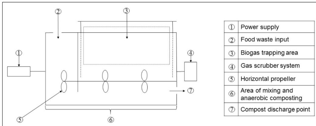
Figure 1. Schematic diagram of pilot-scale anaerobic composter
