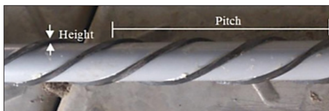
Figure 1. Schematic diagram of cylinder pipe with three-start helical strakes
