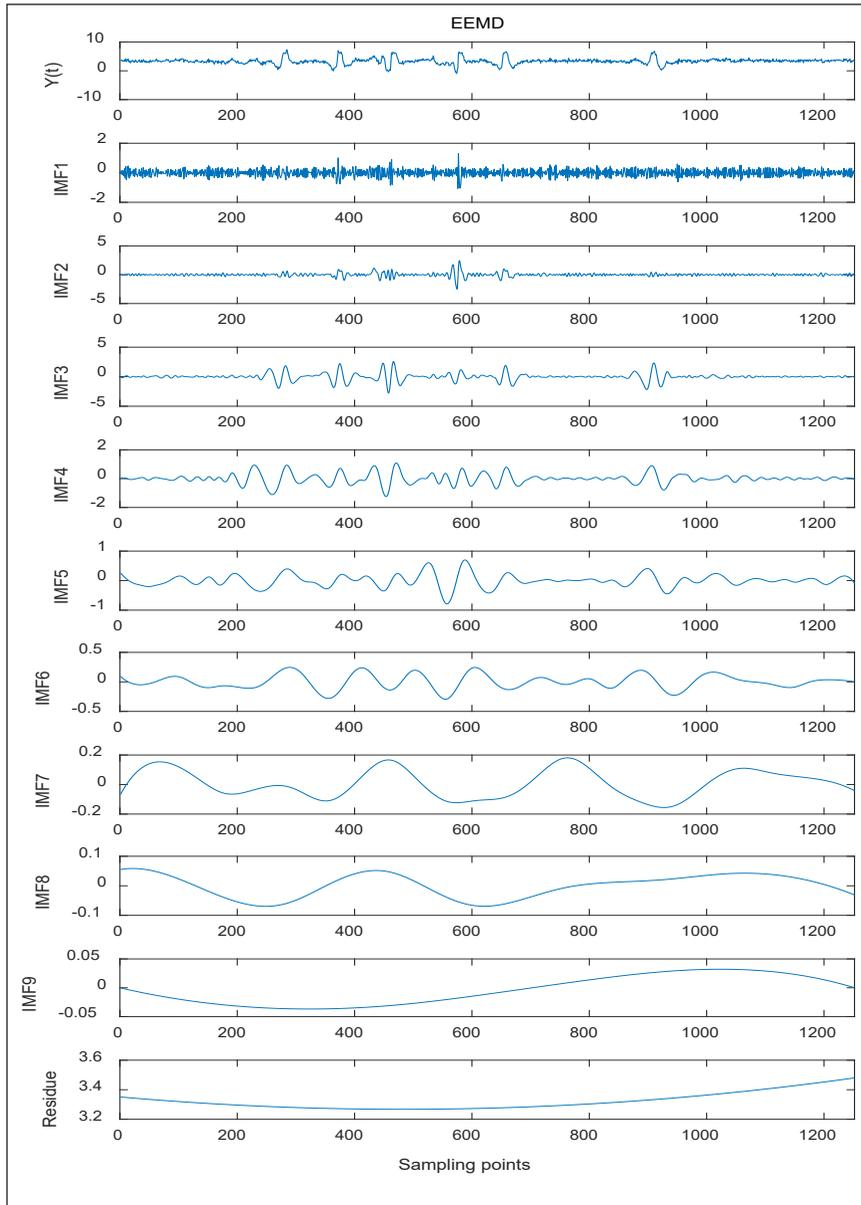
Figure 2. EEMD decomposition of original signal  $Y(t)$
