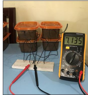
Figure 2. Stacking of four soil-based SMFCs
