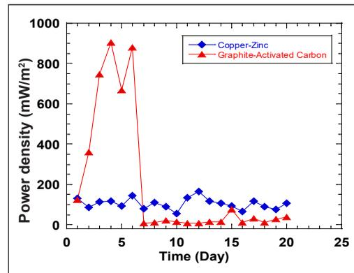
Figure 4. Generated power density of different electrode's material
