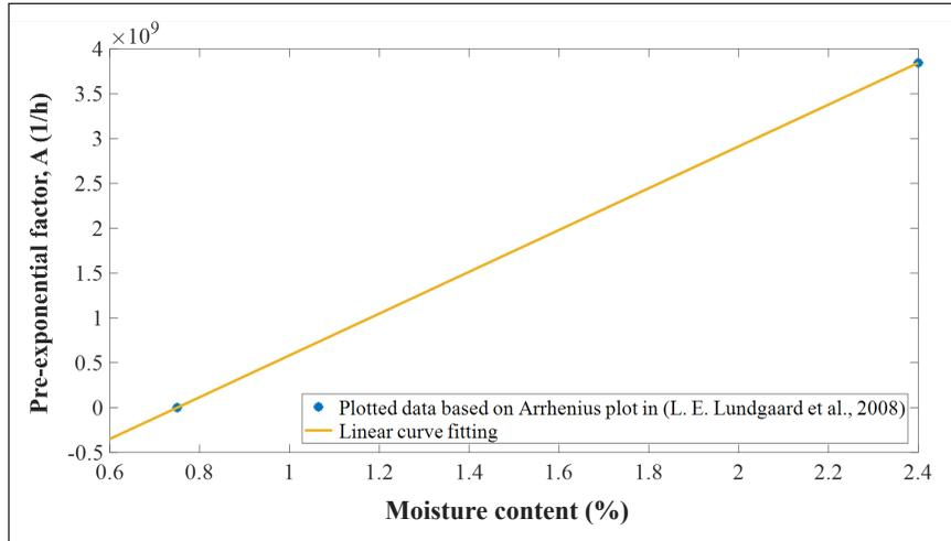
Figure 5. Relationship between pre-exponential factor and LMA/moisture content
