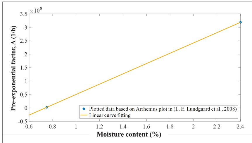
Figure 6. Relationship between pre-exponential factor and HMA/moisture content
