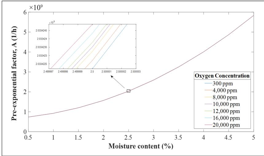
Figure 9. Relationship between pre-exponential factor and moisture content/oxygen/LMA
