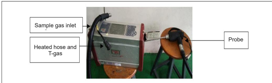
Figure 9. Exhaust gas analyzer
