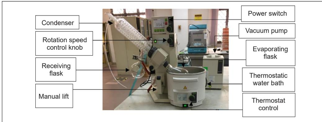
Figure 3. The full set of BUCHI rotary evaporator
