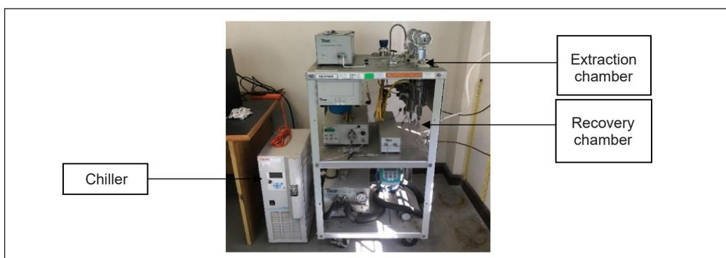
Figure 2. Super Critical Fluid Extraction (SCFE)
