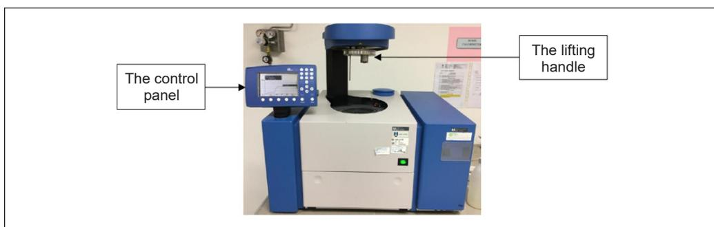
Figure 7. C200 Bomb Calorimeter
