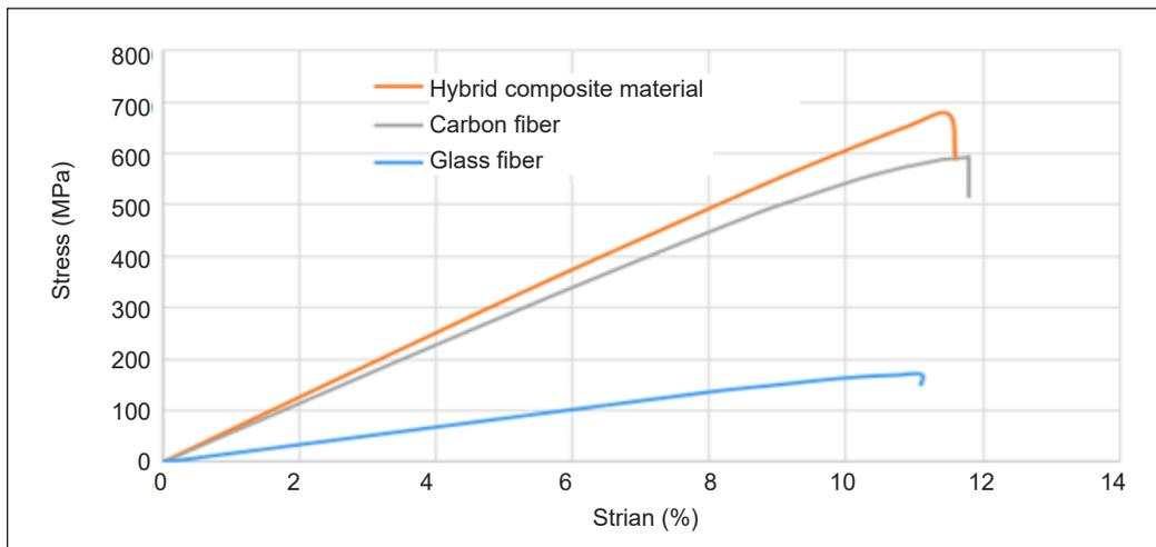
Figure 12. The stress-strain curve of the three tested materials
