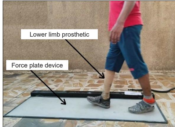
Figure 10. The patient with a transtibial amputee walked on the force plate device
