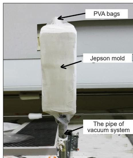
Figure 3. The Jepson mold at the stand of the vacuum pressure to lay up the layers of fibers
