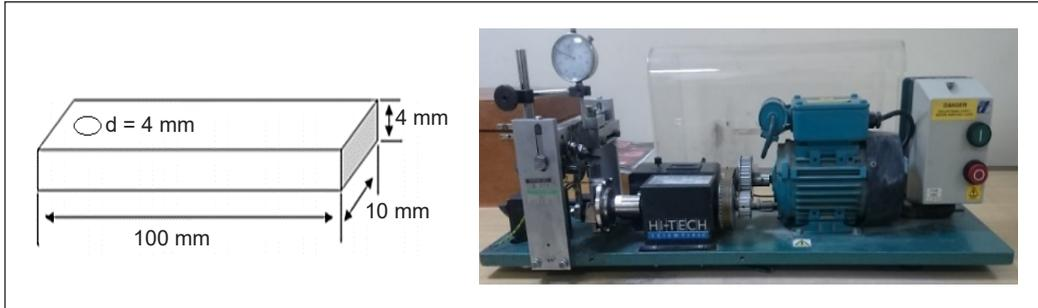
Figure 7. The fatigue test specimen's dimensions with a fatigue machine (HI-TEICH)
