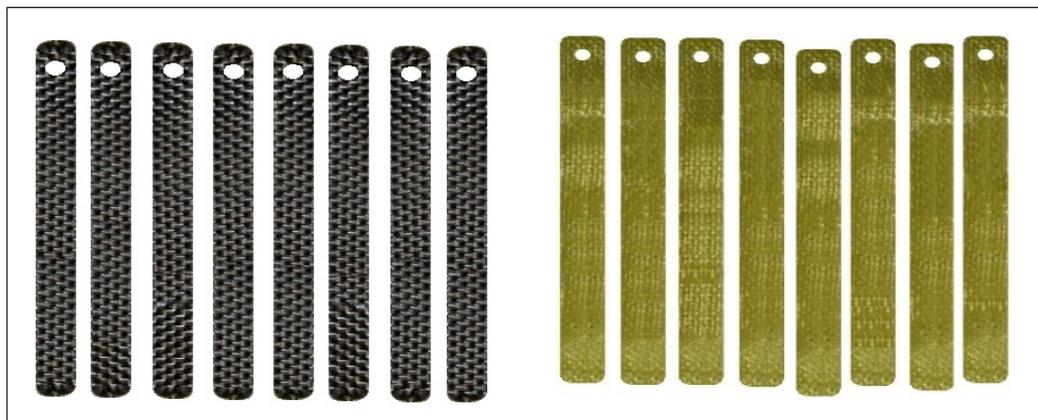
Figure 8. The fatigue specimens of carbon fibers and fiberglass
