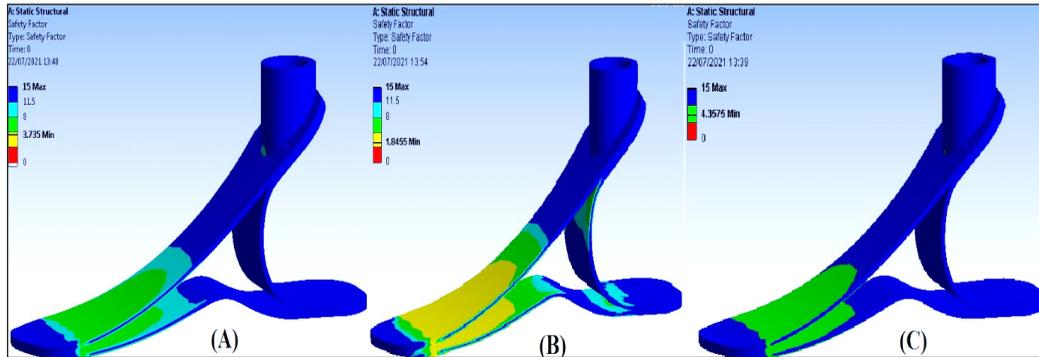
Figure 19. (a) The safety factor value for carbon fiber reinforced foot model at the heel strike stage; (b) The safety factor value for fiberglass reinforced foot model at the heel strike stage; (c) The safety factor value for hybrid material reinforced foot model at the toe-off stage
