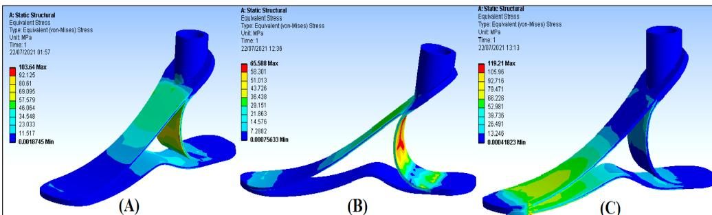
Figure 16. (a) The foot model's Von Mises stress at the heel strike stage; (b) The foot model's Von Mises stress at the midstance stage; (c) The foot model's Von Mises stress at the toe-off stage
