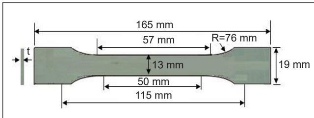
Figure 4. The ASTM D638 dimensions of tensile specimen
