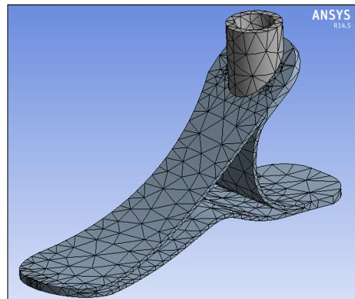
Figure 11. The mesh of the foot prosthetic model
