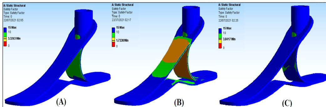
Figure 17. (a) The safety factor value for carbon fiber reinforced foot model at the heel strike stage; (b) The safety factor value for fiberglass reinforced foot model at the heel strike stage; (c) The safety factor value for hybrid material reinforced foot model at the heel strike stage
