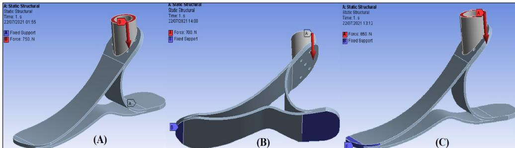
Figure 15. (a) The prosthetic foot model's boundary condition at heel strike position; (b) The prosthetic foot model's boundary condition at midstance position; (c) The prosthetic foot model's boundary condition at the toe-off position
