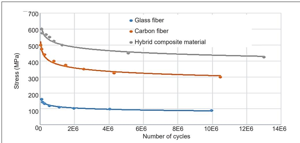
Figure 13. The S-N curve of the three tested materials
