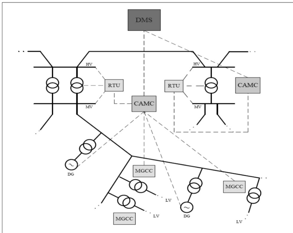
Figure 2. Multi-microgrid control architecture (Lopes et al., 2013)
