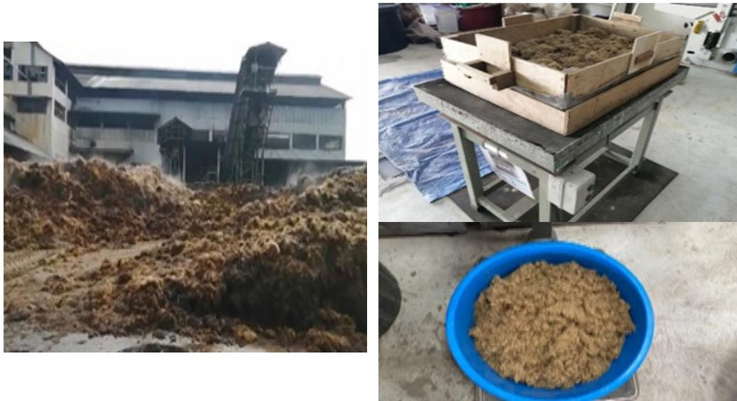
Figure 1. Preparation of fibre from raw to processed fibre
