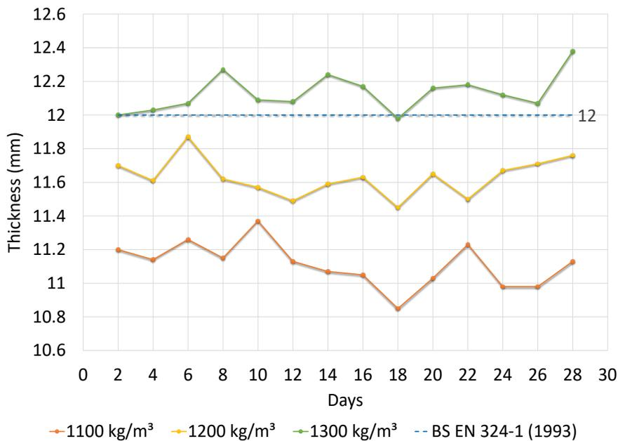
Figure 3. Thickness monitoring of EFBCB for 28 days
