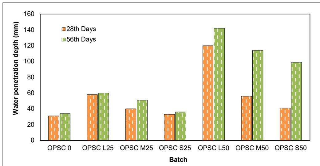
Figure 14. Water penetration test at 28 days and 56 days
