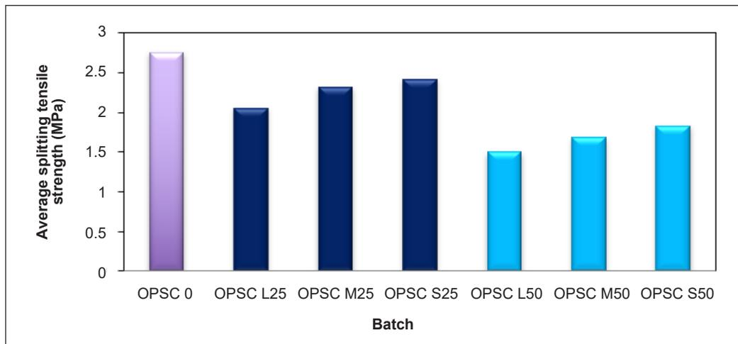
Figure 8. Average splitting tensile strength at 28 days
