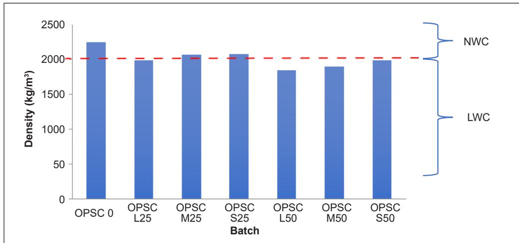
Figure 3. Average concrete density at 28 days
