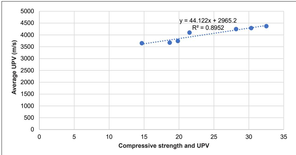
Figure 11. Relationship between compressive strength and UPV
