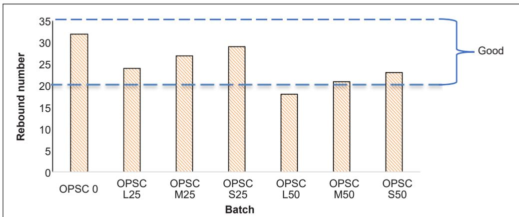
Figure 12. Average rebound number of concretes at 28 days
