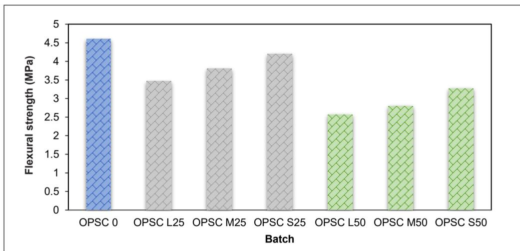
Figure 9. Average flexural strength at 28 days
