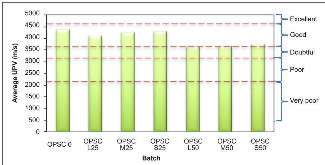
Figure 10. Average UPV of concrete at 28 days
