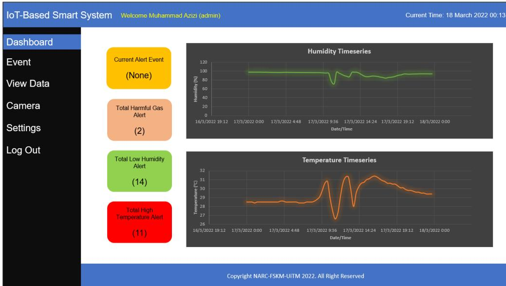
Figure 5. System web dashboard interface
