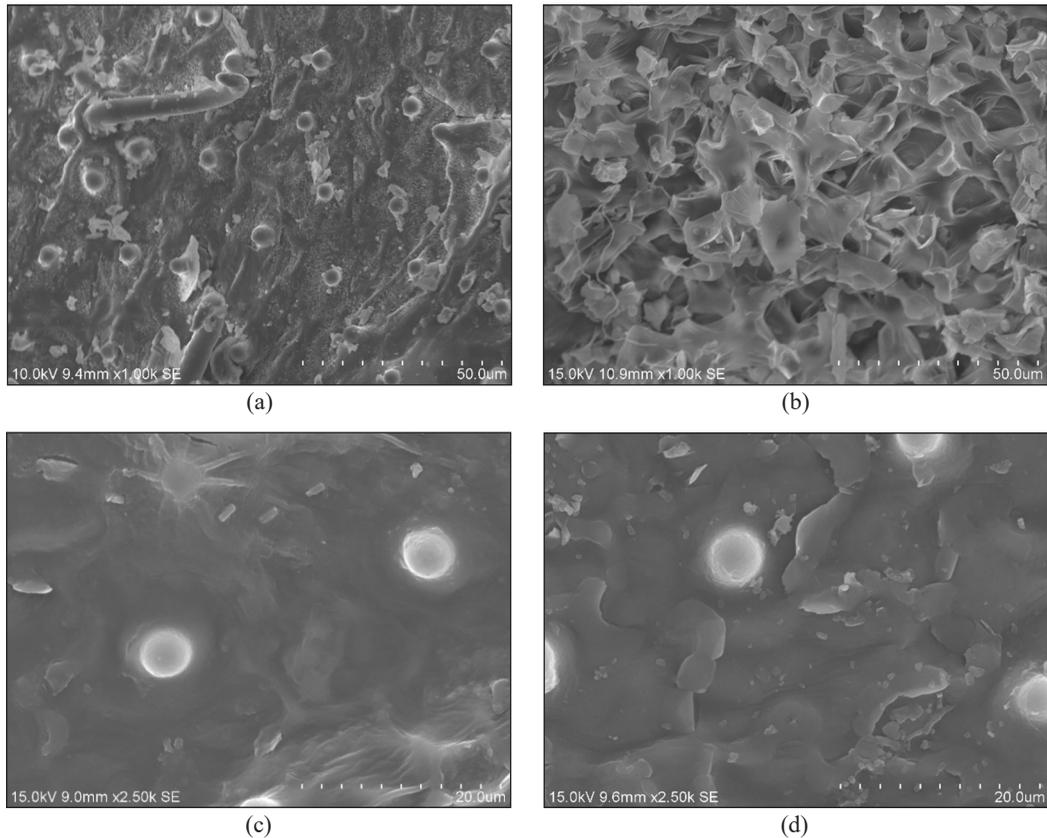
Figure 3. SEM images of (a) sample D before SC-CO<sub>2</sub> extraction, (b) sample D after SC-CO<sub>2</sub> extraction, (c) sample M before SC-CO<sub>2</sub> extraction, and (d) sample M after SC-CO<sub>2</sub> extraction. Note. Sample D: dry sample which undergoes drying and grinding processes; sample M: microwave pre-treatment sample using fresh leaves without drying and grinding processes
