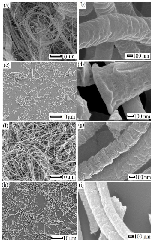
Figure 4. SEM images of sonicated (a and b), untreated PLLA  $t = 29$  min (c and d), UV-Ozone irradiated PLLA  $t = 29$  min (e and f), untreated PAN,  $t = 18$  min and UV-Ozone irradiated PAN,  $t = 18$  min (g and h)
