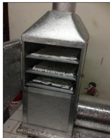
Figure 3. Hot air drying of copra (Pestaño & Jose, 2016)
