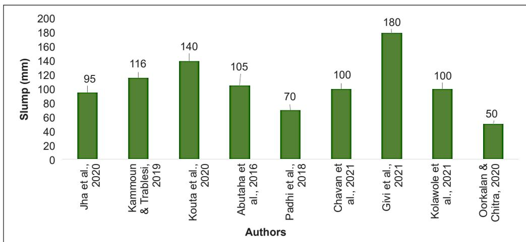
Figure 5. Maximum slump result from different studies
