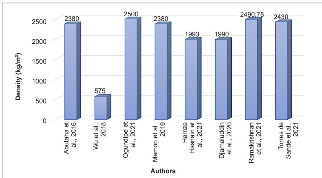
Figure 6. Maximum bulk density results from different studies
