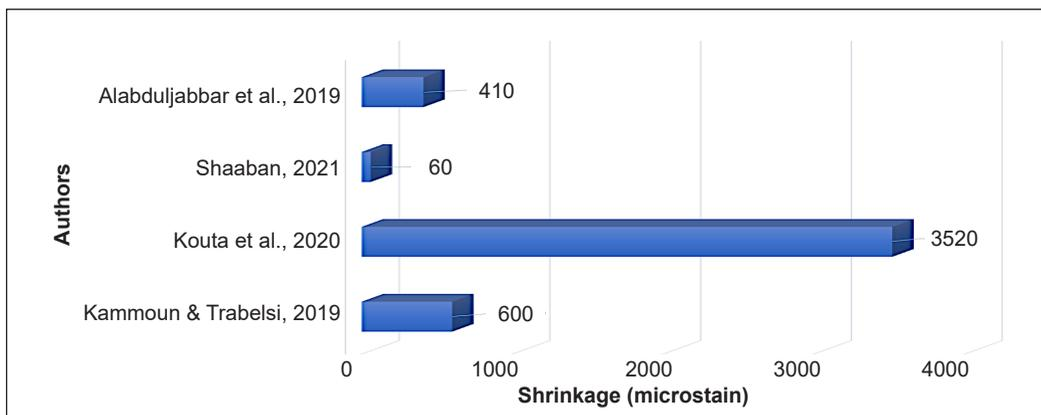
Figure 7. Maximum shrinkage results from different studies
