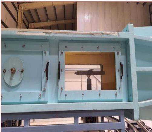
Figure 12. 3D printed model in the test section
