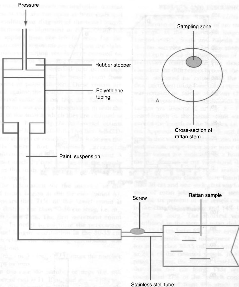
Fig 1. Schematic diagram of the apparatus used to infuse alkyd-paint into a rattan sample. A: The paint applicator is tapped into the shaved end near the periphery of the rattan stem for random sampling
