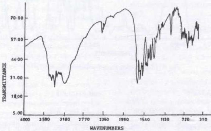
Fig. 5: IR-absorption spectra of 2-amino-6-hydroxy-8-chloroethyl purine (Guanine)
