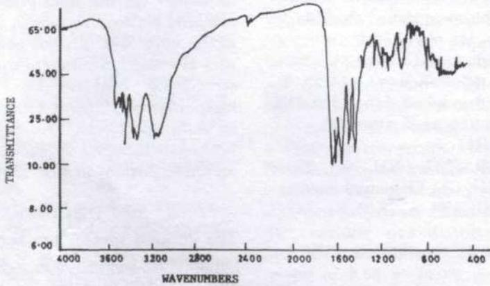
Fig. 3: IR-absorption spectra of 2,6 - diamino-8-chloropropyl purine
