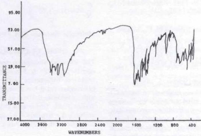
Fig. 1: IR-absorption spectra of 2,6 - diamino-8-chloromethyl purine
