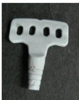
Fig. 6(a): Coated implant using EPD
