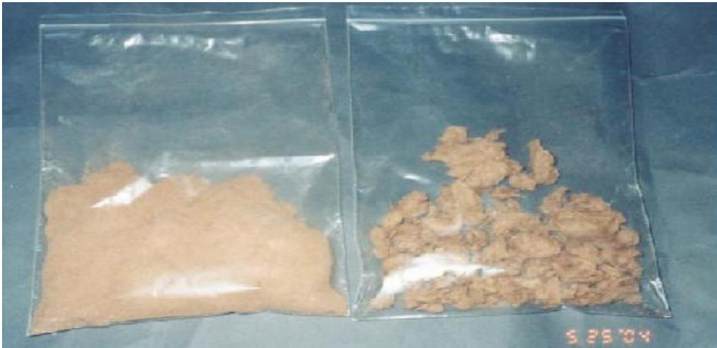
Fig. 2. Fibres from two cycles (2.5-mm plate gap followed by 0.5-mm) of refining (left) and Lumpy fibres from one cycle (0.5-mm plate gap) of refining
