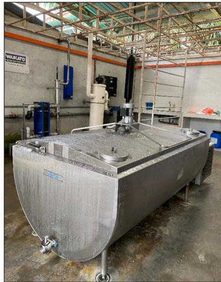
Figure 3. Mueller Model U Open Tank
